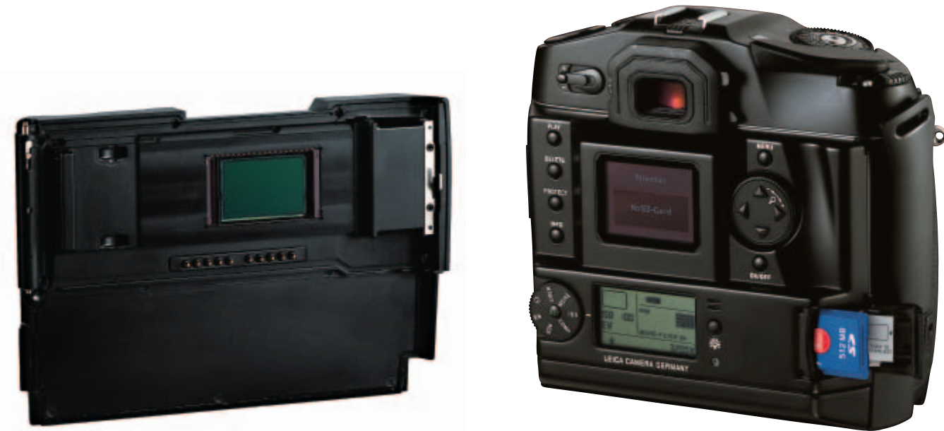
Unlike many other digital cameras, the Digital Module R's sensor has a protective layer that can be cleaned with a standard lens cloth
