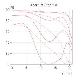
At aperture 2.8 the overall contrast is visibly improved as is the quality in the outer zones of the image. The very fine detail however has a softer definition.
