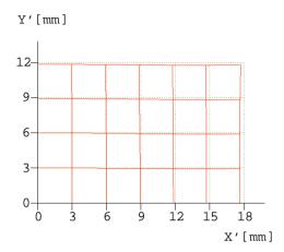
The distortion is 2% and visible in critical situations, but one should not confuse distortion with converging perspective lines.
