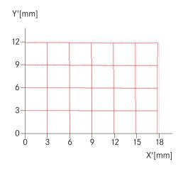
The distortion of the Summilux-R is visible with 2%.
