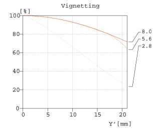
Vignetting is acceptable with 1.8 stops and will not be disturbing in most cases.
